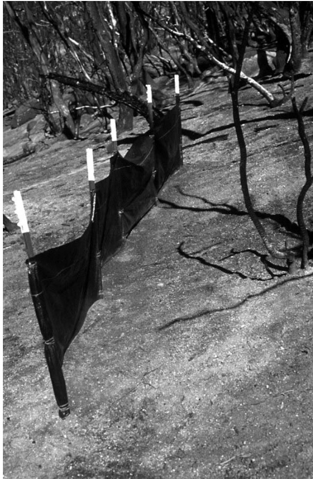
Figure 2. Photograph of a silt fence to measure surface erosion
