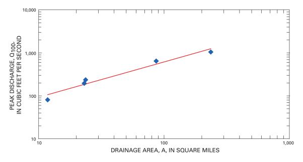
Figure 2–1. Relation of 100-year flood peaks and drainage area showing the best-fit regression line using an ordinary-least-squares regression model.
