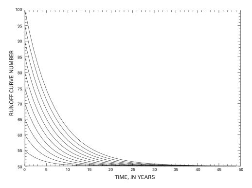
**Figure 3.** Estimated recovery curves for runoff-curve numbers in a drainage basin with a pre-burn runoff-curve number of 50. Plotted curves represent estimated post-burn response of runoff-curve numbers 55 through 100, incrementing by 5.
