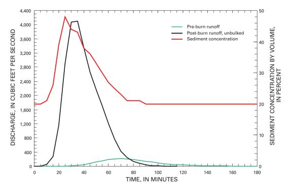
**Figure 2.** Example of pre- and post-burn runoff hydrographs and sediment-concentration hydrograph used in debris-flow modeling, 100-year, 1-hour storm.
