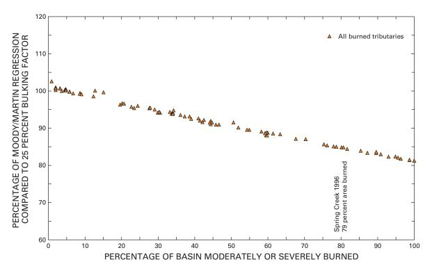
**Figure 7.** Comparison of post-fire runoff sediment-bulking methods, as a percentage of results from Moody and Martin's (2001a) Spring Creek regression on total drainage-basin area to a 25-percent bulking factor applied to moderately and severely burned areas compared to percentage of drainage basin moderately or severely burned.
