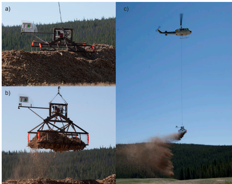
Figure 2. The prototype Heli-Claw being used for wood shred mulching at the Beal Mountain mine site: (a) picking up a load, (b) taking off with the claws closed on a load, (c) applying mulch by opening the claws while flying over the target area.
