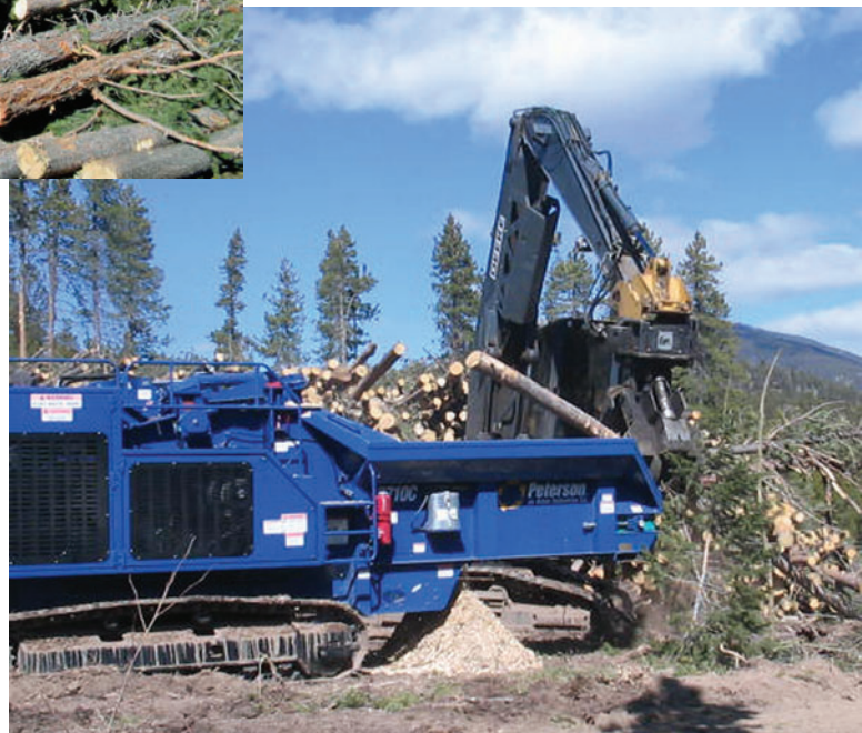
Figure A2. Peterson horizontal grinder.
