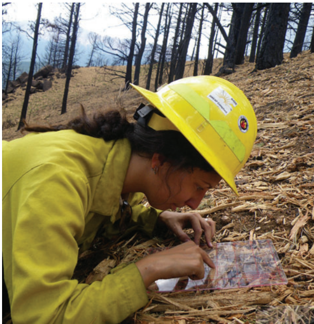
Figure B3. The WoodStraw® grid (Forest Concepts, LLC) being used to sample ground cover for contract compliance during treatment implementation at 2012 Waldo Canyon Fire.
