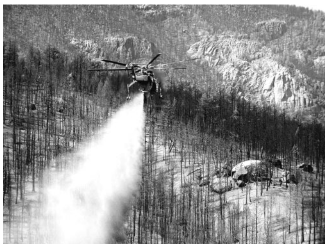
Fig. 5. Aerial application of hydromulch on a research catchment in the high-severity burned area of the 2002 Hayman Fire (Colorado, USA).
