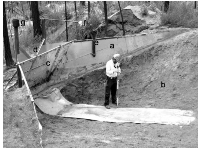
Fig. 1. Typical paired catchment sediment basin after removal of sediment. (a) Sheet metal barrier wall; (b) sediment basin area; (c) debris collection rack; (d) V-notch weir; (e) magnetic/electronic stage sensor; (f) ultrasonic depth sensor; and (g) tipping-bucket rain gauge.
