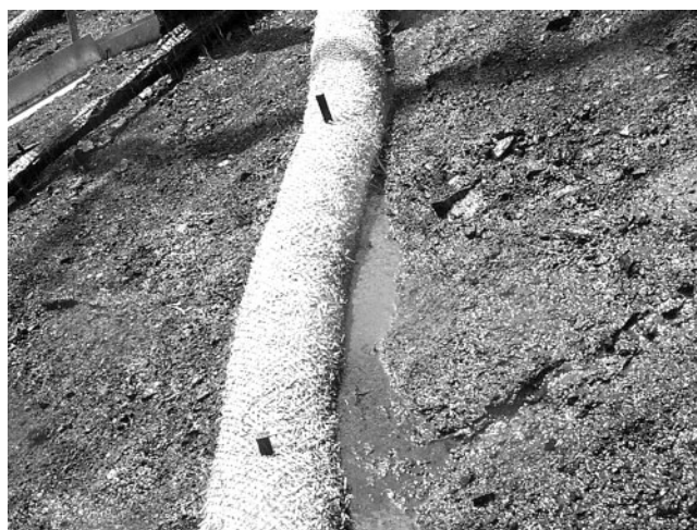
Fig. 6. A straw wattle erosion barrier is tested during a rainfall simulation experiment following the 2000 Valley Complex Fire (Montana, USA).
