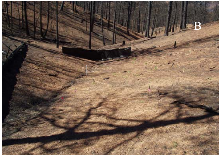
Figure 2. Sediment fence on: (a) a planar hillslope in the Hayman fire in September 2003, fifteen months after burning; and (b) a convergent swale in the Schoonover fire in September 2002, three months after burning.
