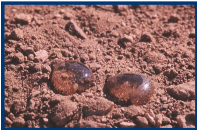
Figure 2.9 —Appearance of water droplets that are “balled up” on a water-repellent soil. (After DeBano 1981).
