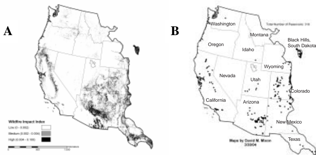
A. Wildfire Impact Index that Includes Effects of Fire Frequency, Soil Erodibility, Channel Slope, And 30-Minute Maximum Rainfall Intensity. B. Location of Only those Reservoirs Within the Black areas in Fig. 1A Where the Wildfire Impact Index is High. Reservoirs Just Outside and Downstream from Some areas With a High Wildfire Impact Index are not Shown.
