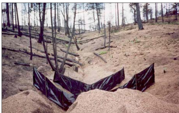
Figure 1. Photo from summer 2003 showing a pair of sediment fences, the piles of sediment excavated from the fences, and the relatively bare hillslopes after the June 2002 Hayman fire.
