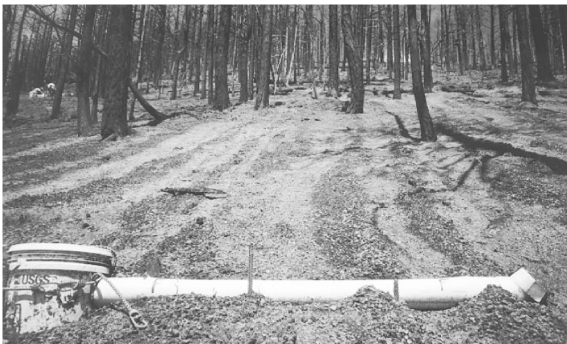
Figure 3. Photograph of rill network that developed above a sediment-runoff trap following the July 16, 2000, storm. View is upslope, and length of the white PVC pipe is 1.5 m
