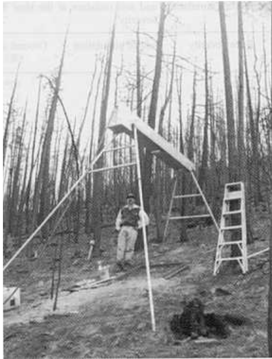
Figure 2. Photograph of the rainfall simulator and runoff plot on a high-severity site in the Bobcat fire
